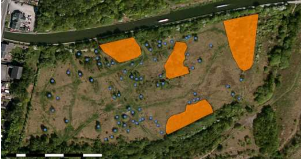
Figure 4: Tree removal works. Individual trees marked in blue, areas of tree removal marked in orange.
